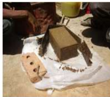
Step 4. Removing block from the mold
