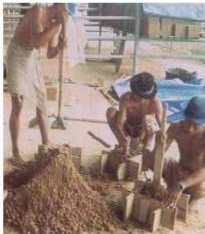
Molding using wooden bars
