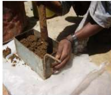
Step 1. Filling the mold
