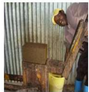
Machine for making solid construction blocks
