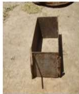
Mold made of metal sheets – Holeta Research Center
