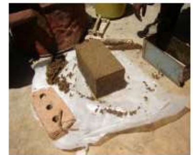
Step 5. UMB ready for drying
